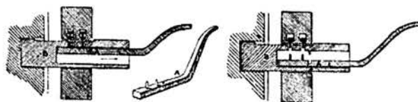
FIG. 2.—EGYPTIAN WOODEN LOCK AND KEY.
