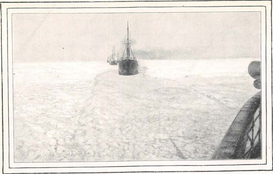
A FLEET OF ICE-BOUND VESSELS BEING CONDUCTED INTO KRONSTADT BY THE "ERMACK." The snow, which lay about a foot deep on the ice, retarded the progress of the ship more than did the ice itself. The picture shows into what fine pieces the "Ermack" breaks the ice.
