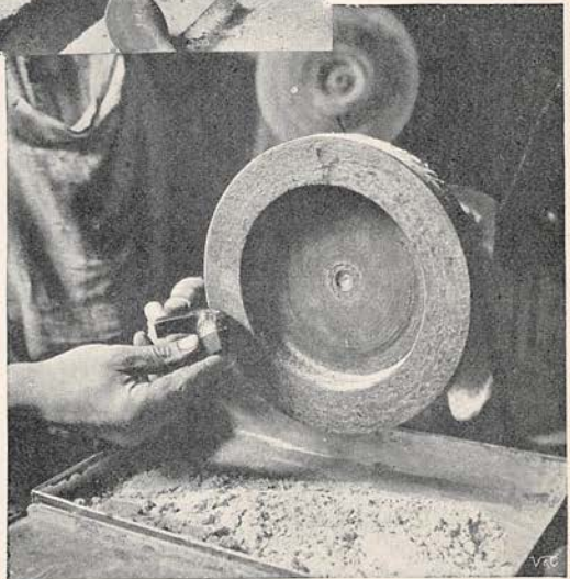
POLISHING WITH POWDERED PUMICE.
