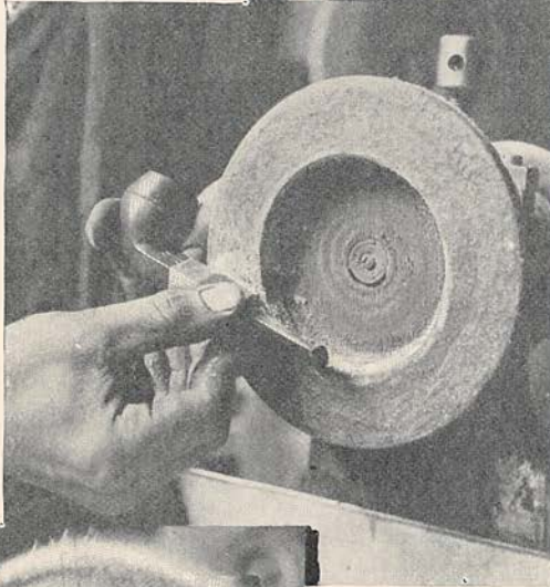
POLISHING WITH POWDERED PUMICE.
