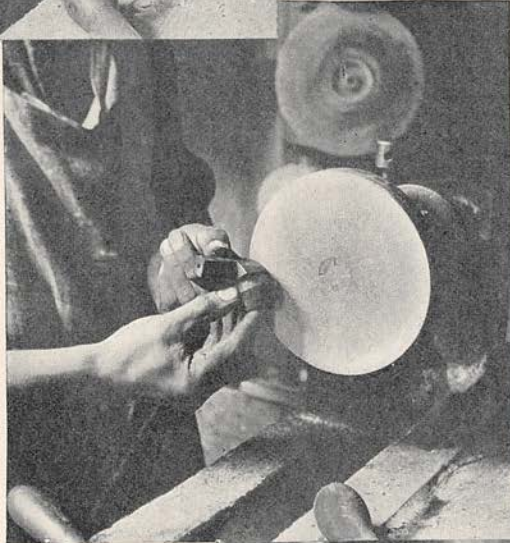
SMOOTHER GRINDING ON STEEL DISC
