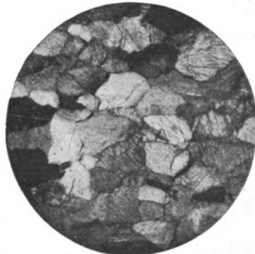
Microphotograph of the Carrara marble after having been slowly deformed during 124 days at a temperature of 300deg. Centigrade. The individual grains can be seen to be flattened in a horizontal direction.
