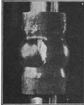
In this case the pressure on the marble was continued so long and the deformation carried so far that the moving marble within rent asunder the metal jacket inclosing it.
