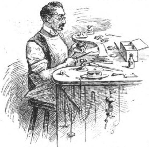
FILING AND DRILLING THE ROUGH CAST.
