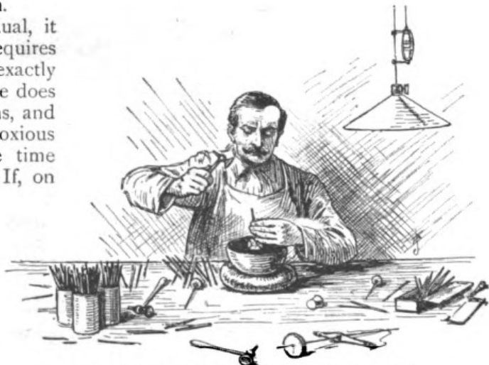
CHASING THE CAST, WHICH IS EMBEDDED IN PITCH.
