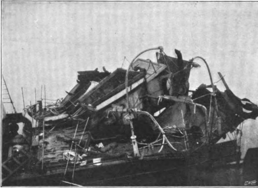
From a] THE FORE-PART OF THE STEAMER AFTER THE EXPLOSION. [Photograph.
