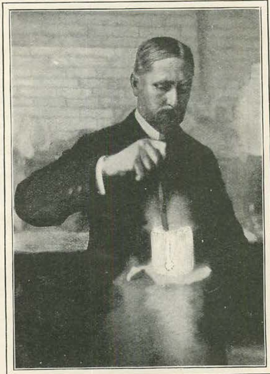
BURNING STEEL IN AN ICE TUMBLER PARTLY FILLED WITH LIQUID AIR. A point of interest in this experiment is the contrast in temperatures; steel is burning at 3,500deg. F. in an ice receptacle containing liquid air at 312deg. below zero.
