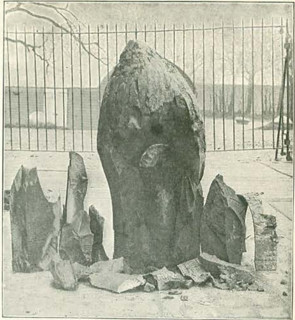
PROJECTILE—AND FRAGMENTS—AFTER BEING FIRED AT ARMOUR-PLATE.
