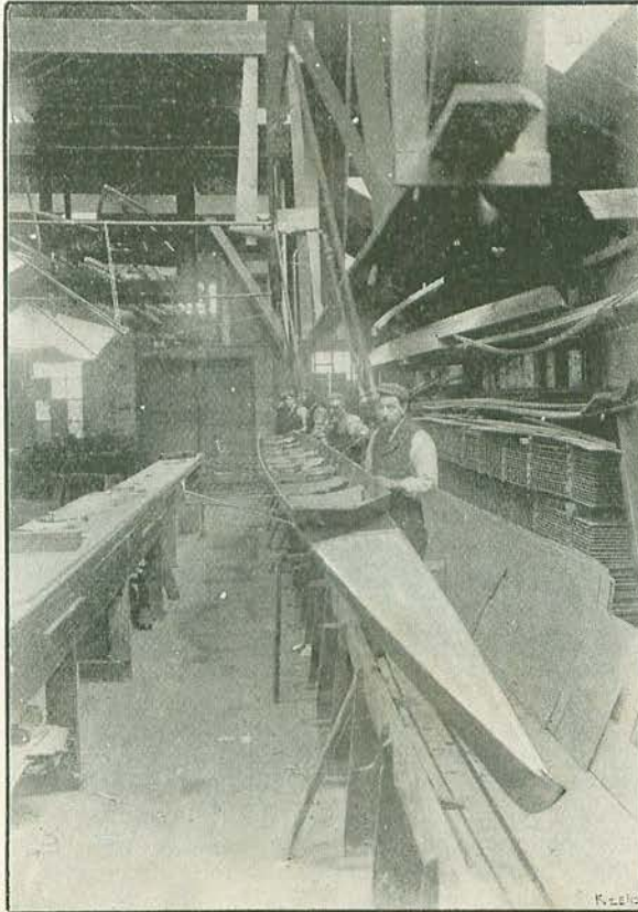
FIFTH STAGE—SHOWING LINEN COVERING, CUTWATER, AND OUTRIGGERS.
