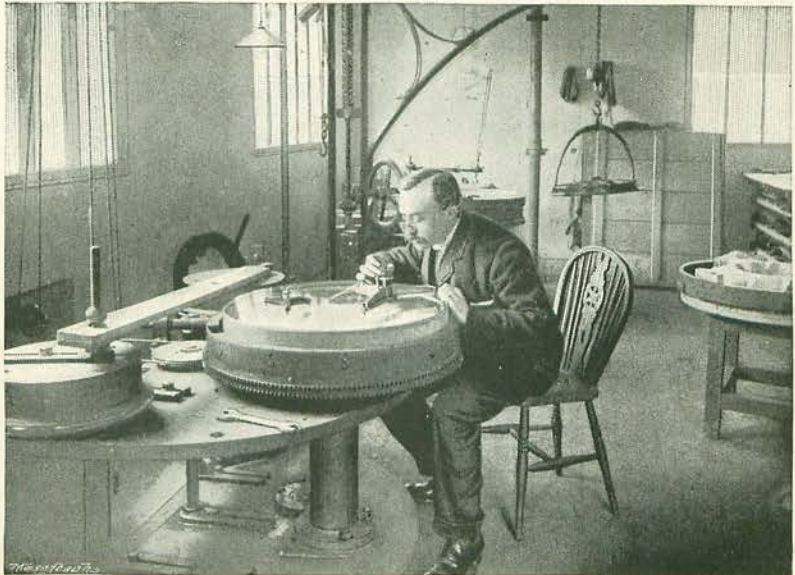
SIR HOWARD GRUBB TESTING AN OBJECT-GLASS. From a Photo. by Sir Howard Grubb.
