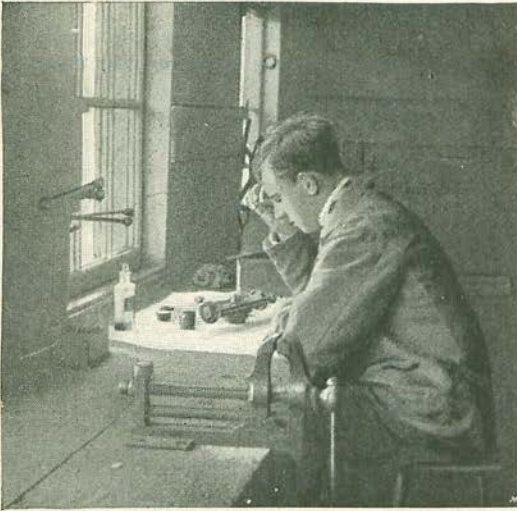
INSERTING THE "SPIDER-LINES." From a Photo. by Sir Howard Grubb.
