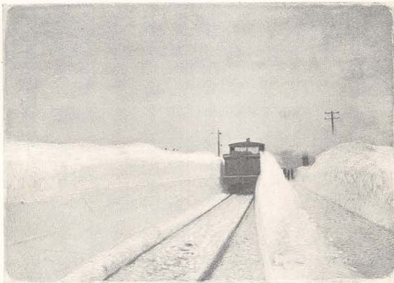
VIEW OF TRACKS FREED OF SNOW, THE CLEAR CUT MADE BY THE ROTARY PLOW, AND THE SNOW AS FORCED BACK BY THE WEDGE-PLOW.
