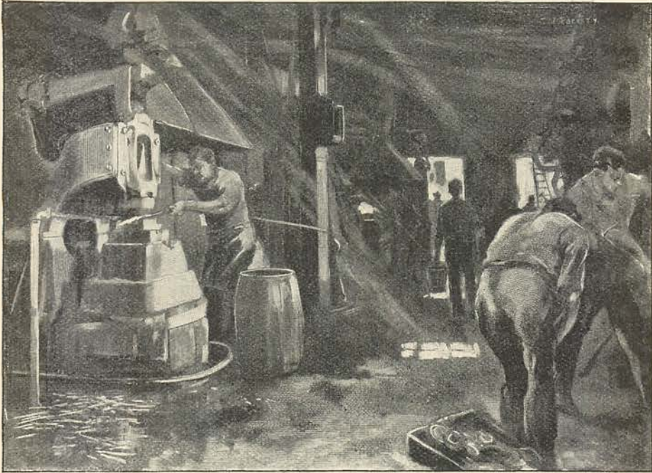
A VIEW OF THE FORGE ROOM, SHOWING ONE OF THE BIG TRIP-HAMMERS, WHICH STRIKE TWO HUNDRED TIMES A MINUTE.
