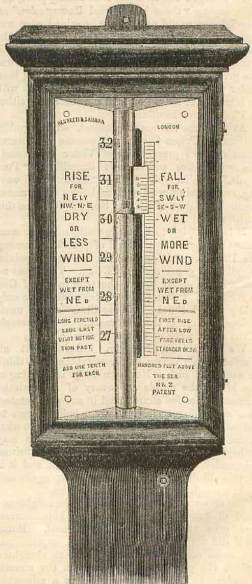
SCALE OF THE BAROMETERS USED AT THE STATIONS OF THE NATIONAL LIFE BOAT INSTITUTION.
