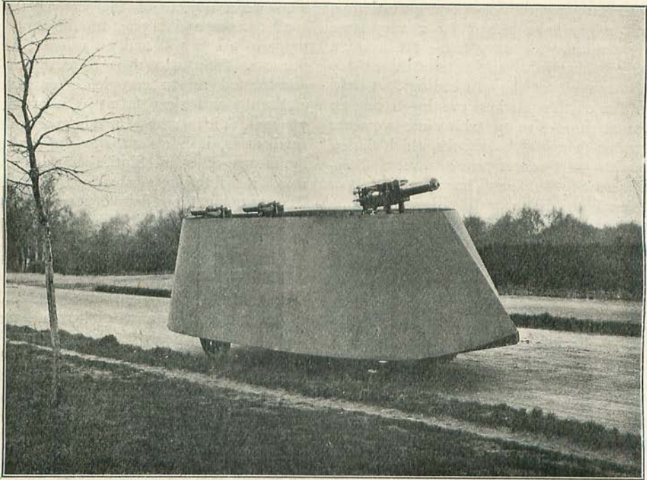
The Simms Motor War-car, showing the armoured rams and poms-poms and maxims
