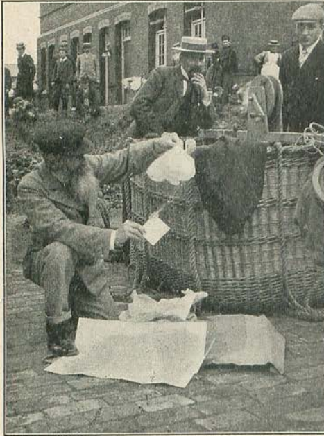
Adjusting the parachute which conveys messages from the balloon to the earth
