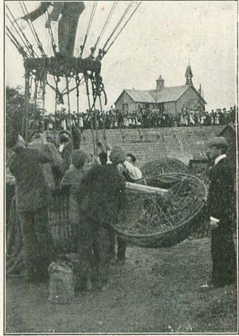
Affixing the collapsing drum to the balloon
