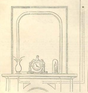
The Air-Syphon Ventilator admits also of being extemporaneously and temporarily set up in a sick-room, so as to cause a constant removal of air from the upper portion of the apartment, where it is so apt to hang about the curtain furniture of the chamber, and to impregnate it with the exhalations which are so often the result and generators of disease.
