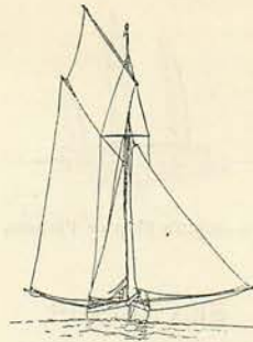
Jib-tack as Sheet. Jib set as Spinnaker or Studding-sail.
