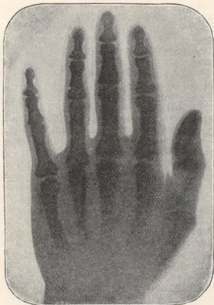
THE LIVING HAND, PHOTOGRAPHED THROUGH BLACK VULCANISED FIBRE, WITH AN EXPOSURE OF FOUR MINUTES.
