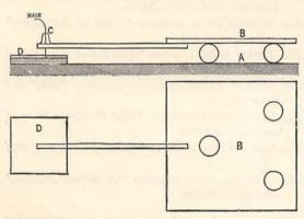
placed level once for all. On this rest three accurately turned ivory balls about 11 inches in diameter, and on the top of these balls is placed a plate, B, similar to the lower, but having attached to it a projecting arm with a long vertical hole pierced through | relation of the famous Munchausen, made a statement
