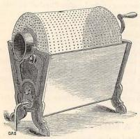
or a quarter of a pound in three minutes. and is remarkably cheap. Being a quick roaster it produces finer coffee than the slower roasters in the trade. The cylinder containing the coffee is turned by the handle shown, and the
