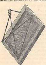
pose the mirror so that it can be most serviceable. American device illustrated in the engraving is an improvement on the old plan which will be found useful in many cases. It is so simple that any skilful metal - worker will be able to construct the parts from the figure. The hookpiece is screwed to the wall, and the mirror or picture can be inclined
