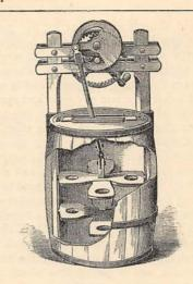
placed on the crank shaft, and worked by an internal gear wheel connected with the lower cross-bar of the frame. Driving power can readily be obtained by placing a pulley on the crank shaft. The churn-cover may be easily removed without interfering with the frame by which it is supported.
