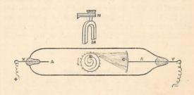
begins to turn, by the impact of the stream on the projecting vanes. On presenting the opposite pole of under side of the wheel, and the rotation first stopped, then reversed. In this way the wheel can be made either "overshot" or "undershot."
