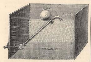
way into even the best-regulated reservoirs. The tap is attached outside near the foot of the cistern, and the flow-pipe within is fastened at its top to the float, and rises and falls with it. All sediment having a natural tendency to sink, it is evident that while the bottom of the cistern will be covered with a layer of the sediment, the water above will remain clear. The water
