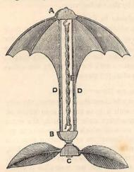
There is a similar hook in B, turning freely therein, but fastened in another piece of cork, C. From hook to hook, and between the rods, a rubber band, E, is stretched; and in the cork, c, two feathers are inserted, like the fans of a propeller.
