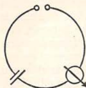
FIG. 3. RESONATOR WITH GALVANOMETER ATTACHED.
