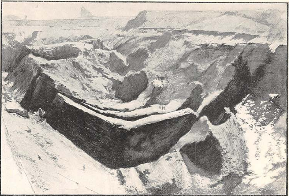
THE «STRIPPINGS» OF A MODERN COAL-MINE, SHOWING THE EXPOSED VEINS OF ANTHRACITE, WHICH VARY FROM FORTY TO SIXTY FEET IN THICKNESS.
