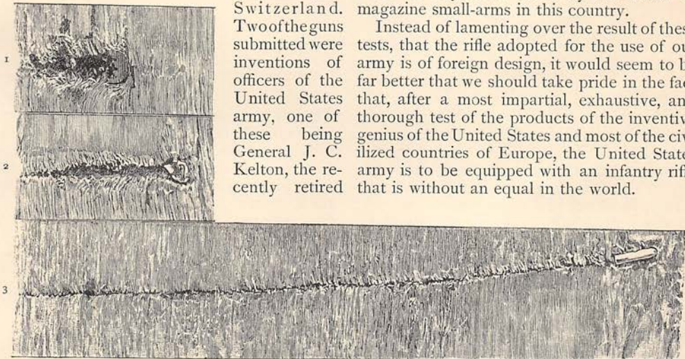
1. PENETRATION IN OAK (3.3 INCHES) OF THE .45-CALIBER LEAD BULLET. 2. PENETRATION IN OAK (5.3 INCHES) OF THE .45-CALIBER GERMAN-SILVERED BULLET. 3. PENETRATION IN OAK (24.2 INCHES) OF THE .30-CALIBER BULLET WITH NICKEL-STEEL JACKET.
