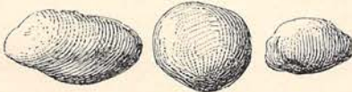
FIG. 8. ROUNDED PEBBLES AND SMALL COBBLESTONES TO BE CAREFULLY EXCLUDED FROM ALL MACADAM AND TELFORD ROAD-MATERIALS.
