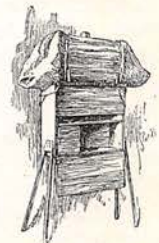
A "HOME-MADE" WET-PLATE OUTFIT.
