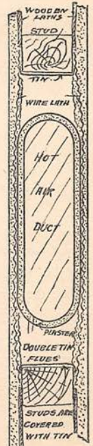
FIG. 10.—HOT-AIR FLUE OR DUCT IN PLASTERED PARTITION.
